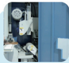
右刀架 RIGHT CUTTER UNIT 90度及45度雙刀架採用油壓系統作動具高度穩定性 Hydraulic control of two cutter unit 90° and 45°, ensuring stability.
